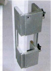
**Rout jambs before you install.** The clamp-around design of this jig won't work with jambs that are already installed.
