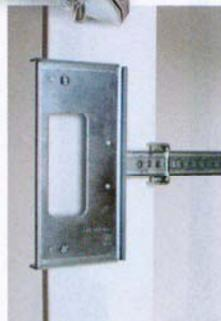
**Tag team.** This is the only two-part jig: one piece for the door hinges and one for the jamb hinges.
