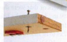
**Loss insurance.** The template nails on this jig are held in place by a nut, so they can't be lost.
